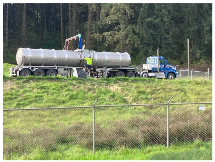
(caption: Leachate tanker truck filling up at Coffin Butte Landfill. With an estimated capacity of 5500 gallons, these tankers make approximately 20 trips per day to Corvallis and Salem.)
